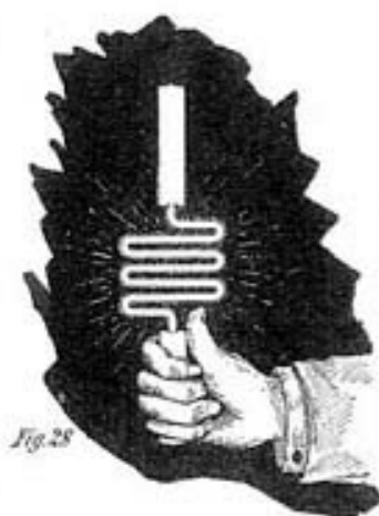
FIG. 28.—INCANDESCENCE OR PHOSPHORESCENCE OF RAREFIED GAS.—ILLUSTRATING FOUR KINDS OF LIGHT EFFECTS PRODUCED BY HIGH FREQUENCY CURRENTS OF HIGH POTENTIAL.
